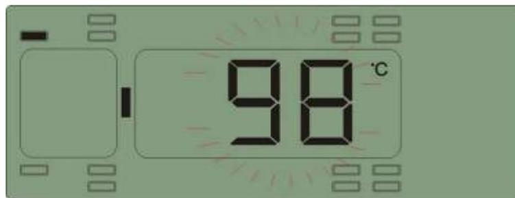
Function: When the temperature around the transmitter equals or exceeds 90°C, the system will issue the high temperature alarm.
