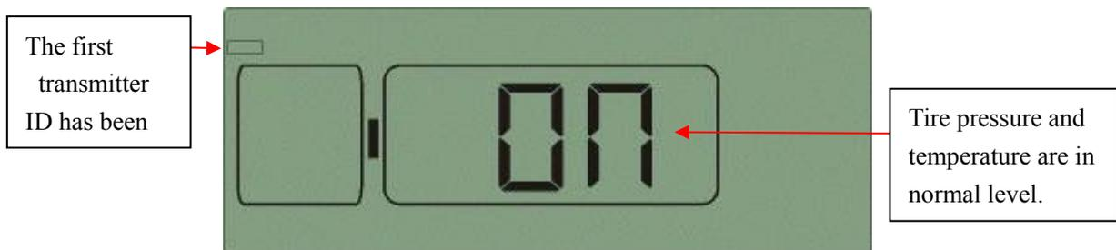
If the above figure is displayed, it indicates that the transmitter is installed correctly and the user can install the next one. When all the transmitters have been installed correctly, screen will display as shown below:
