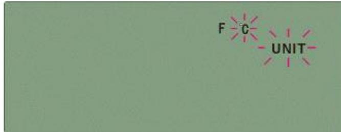
Press up or down arrow key to choose temperature unit which will flash, the “UNIT” will flash all the time indicating that the present interface is not the inquiry but the programming interface as shown below:
