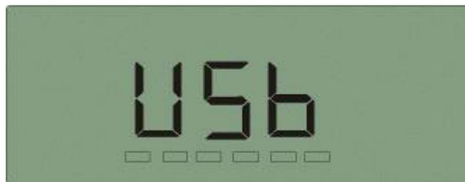
Now system is in the mode waiting for information uploading, and all the buttons can not be used until the USB cable is pulled out. Connect the other end of the USB cable to computer, and then open the Monitor Log receiving software in the computer. Click the upload button of the software, monitor will upload the data as shown below:
