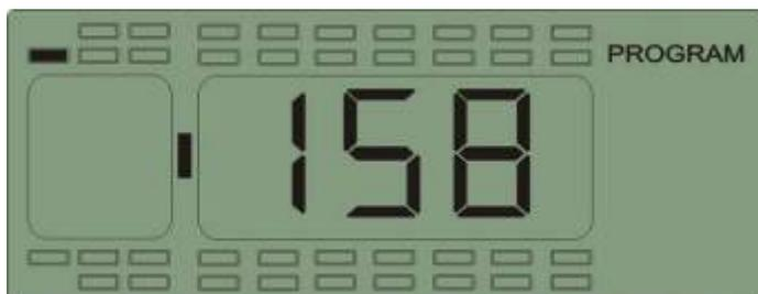
6. When finish programming these 3 digits, press S for 3 seconds to save with the screen flashes twice, beep buzzes twice. Then it will automatically switch to next tire position.
