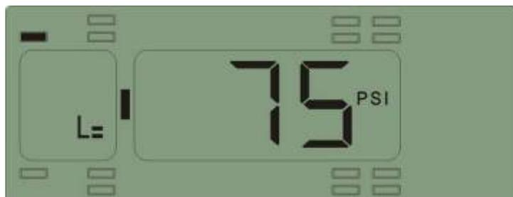
Function: The system will issue level 2 low pressure alarm when the tire pressure is 15% lower than the standard pressure.
