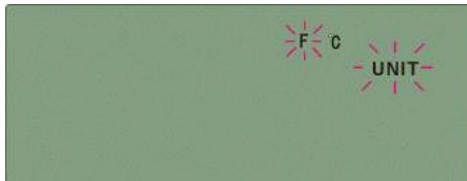
Then press S for 3 seconds to save with beep buzzes twice. All the icons will stop flashing and only the selected unit is displayed.
