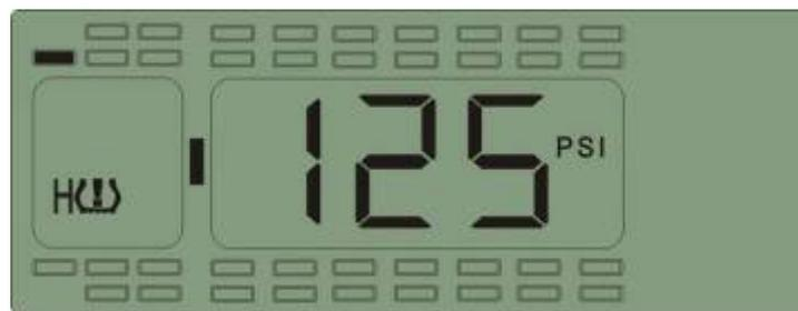
Function: The system will issue the high pressure alarm when the tire pressure is 25% higher than the standard pressure.
