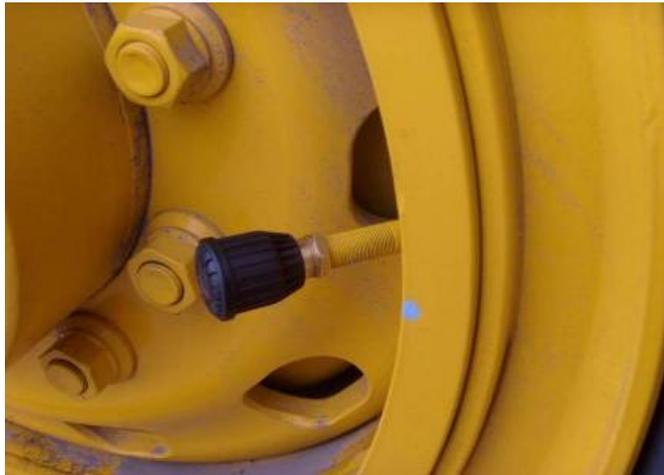
6. Check the connection of transmitter and valve with the soap solution to confirm whether the transmitter is firmly screwed onto the valve or not, check whether there is air leakage caused by the installation or the seal of the transmitters or not.
