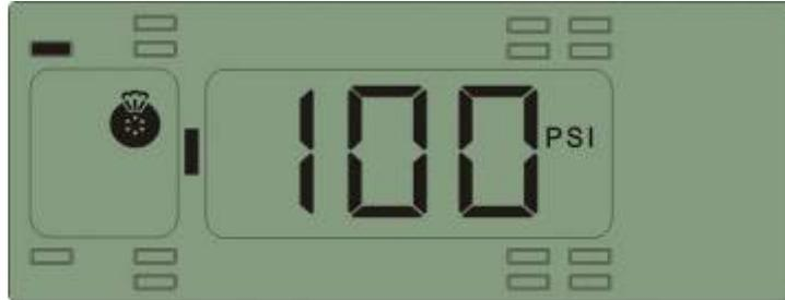
Function: The system will issue a fast leak alarm when the pressure drops more than 0.20BAR within 12 seconds.
