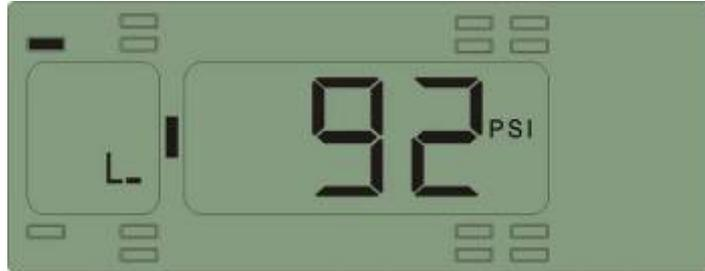
Function: The system will issue level 1 low pressure alarm when the tire pressure is 10% lower than the standard pressure.
