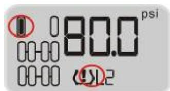
Function: The system will issue a Low Pressure Level 2 Alarm when the tire pressure is 25% lower than the standard.
