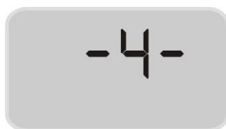
Under the deletion interface, hold and press S key for 3 seconds to return to interface 4.
