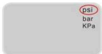
Under the pressure unit inquiry state, hold and press E key for 3 seconds to enter the programming interface. The current unit will continue to flashes as the red part in the picture.
