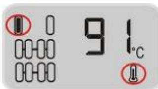
Function: The system will issue a High Temperature Alarm when the temperature around the tire valve exceeds 90°C.
