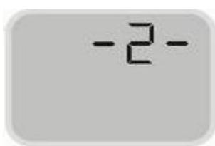
Under the standard pressure inquiry interface, hold and press S key to return to the programming interface 2.
