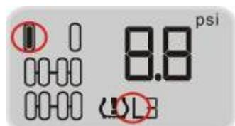
Function: The system will issue a Low Pressure Level 3 Alarm when the tire pressure is 50% lower than the standard.
