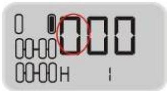
Under the ID inquiry interface, hold and press E key for 3 seconds to enter the ID programming interface. At this time, the first digit on the left starts to flash, press S key to adjust the value from 0~9.
