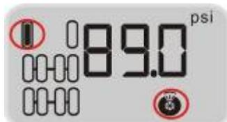
Function: The system will issue a Quick Leak Alarm when the pressure drop exceeds 3psi within 12 seconds.
