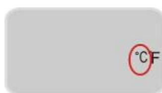
Under the temperature unit inquiry state, hold and press E key for 3 seconds to enter the temperature unit programming interface. The current temperature unit continues to flash as the red part in the picture.
