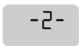
Under the normal mode, press E key for 3 seconds to enter into the programming interface, press S key to switch to programming interface 2.
