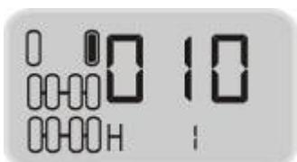
Program all the 12 ID at the H1,H2,L1,L2 positions, hold and press E key for 3 seconds to save the programmed ID with beep buzzes twice, and then return to the ID inquiry interface. Press S key during the process of programming will drop the current operation and return to the ID inquiry interface.
