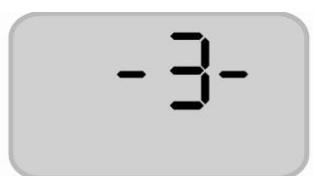
Under the normal mode, hold and press E key 3 seconds to enter the programming interface, then press S key to switch to the programming interface 3.
