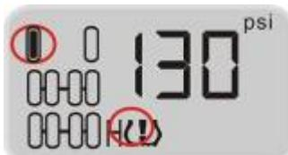
Function: The system will issue a High Pressure Alarm when the tire pressure is 25% higher than the standard.
