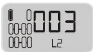
Press S key to switch ID display, at this time the screen display the second low 3 ID, the “L2” stands for the current display.
