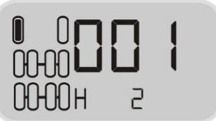
Press S key to switch ID display, at this time the screen display the second high part, the “H2” stands for the current display.
