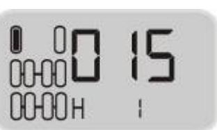
Under the interface 1, press E key to enter the Transmitter ID inquiry and programming interface. It will first display the first 3 ID digits (or the first high part) of Transmitter on the front left tire, the “H1” on the screen stands for the current display.
