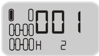
Press S key to switch ID display, at this time the screen display the low 3 ID, the “L1” stands for the current display.
