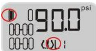
Function: The system will issue a Low Pressure Level 1 Alarm when the tire pressure is 12.5% lower than the standard.
