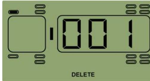
2. Press any of the four arrow keys to locate the tire position to be deleted.
