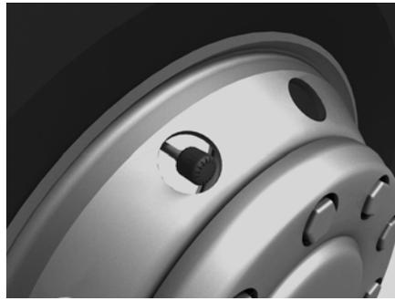
1. Remove the current tire valve cap.
