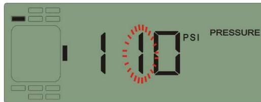
5. Once finished programming the second number, press
