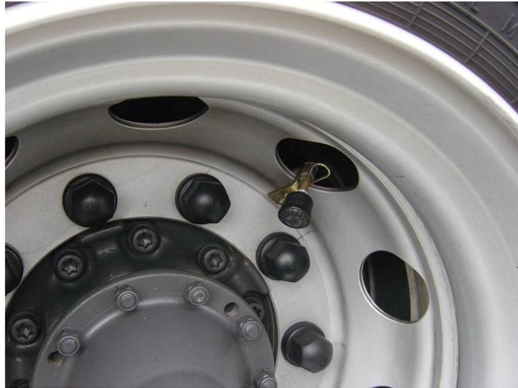
1. Remove the current tire valve cap.
